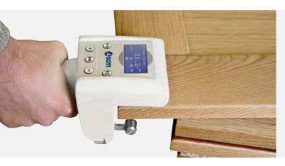
The wireless electronic gauge allows the machine to be positioned at the work thickness measured by the device. The communication with the machine is wireless and the working program can also be launched from the remote control.
