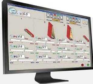
The "PWM" system is totally managed by the "MAESTRO PRO-SAND" electronic control. Thanks to the advanced operator interface developed specifically by SCM, all the device parameters can be displayed, set and saved in each work program.
