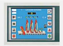
The "PRO-SAND" control is used to set all the operating parameters on the touch screen, and to check in real time the correct operation of the machine.
