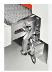
Automatic feed belt centering system: an electro-pneumatic system keeps the feed belt in the best conditions of use at all times without any operator's intervention.
