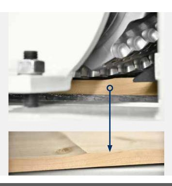
The heavy **sectional presser**, fitted with an anti-kickback safety device, ensures **efficient**, **safe workpiece feed** and also makes it possible **to process parts of different thickness at the same time**.
