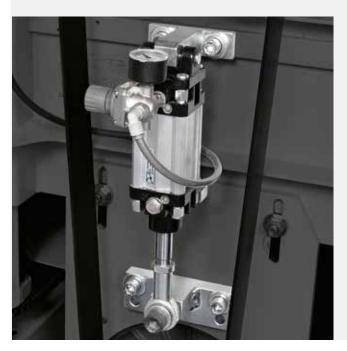
The calibrating/sanding rollers are equipped with an automatic belt tensioning system which allows to keep constant at the correct tension the belt and ensures the maximum efficiency of the power transmission.
