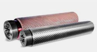
The grooved-steel roller ensures the maximum precision when calibrating solid wood, even when the wood is knotty or has an irregular grain. The hardness available range (from 85 to 20 Sh) for the rubber-coated roller, ensures excellent results on any type of operation, from calibrating with high rates of stock removal to the finishing of veneered and painted panels.
