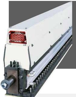
The **"EPICS"** sectional pad consists of a special monolithic beam which houses the cylinders that activate the independent sectors. Thanks to the wide excursion of the pistons and the double action system (adjustable pneumatic push/counter push), the "EPICS" pad guarantees maximum sensitivity and precision in any type of machining.
