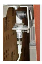
The centering system of the abrasive belt is managed by a very reliable and precise "background suppression" photocell ensuring the correct positioning of the abrasive belt.
