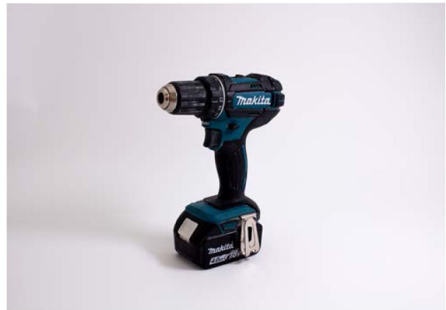
2. Screw gun To fix the acoustic boards mechanically
