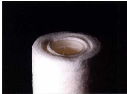
Poor End Sealing & Bypass
