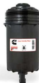
The high performance Fleetguard Filter-in-Filter technology for High Pressure Common Rail engines provides optimally designed filter media to prevent water-related corrosion in modern high pressure fuel systems. The filter features two-stage particle removal with a 5 micron filtration rating and eliminates the hassle of extra filters and fuel plumbing. Its unique design allows reuse of the filter canister and replacement of only the filter cartridge at service time.
