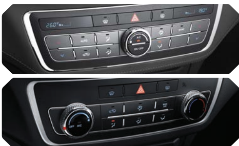
Automatische dual-zone airco / Manuele airconditioning
