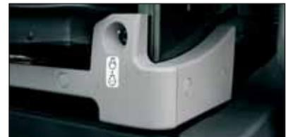
Pilot control shut-off lever
