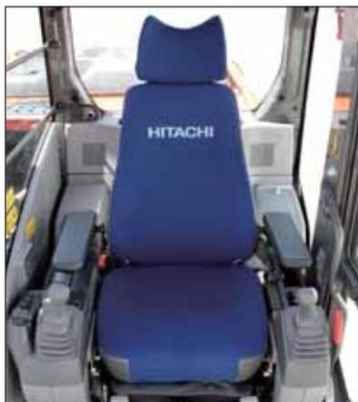
Wide adjustable armrests and a retractable seat belt are included. Short stroke levers allow for continuous operation with less fatigue. Three switches on the lever (optional) can be set to operate attachments other than buckets. The cab is pressurized to keep out dust. Noise and vibrations are kept to a minimum due to the elastic mounts, filled with silicone oil, the cab rests on.
