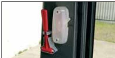
Engine shut-off switch
