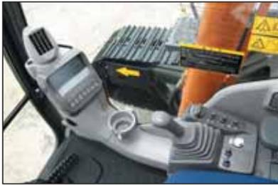
The color LCD monitor, located in the cab, indicates coolant temperature, fuel level, and maintenance data. It also allows one-touch adjustment of the attachment. The display can also be adjusted to day or night shift.
