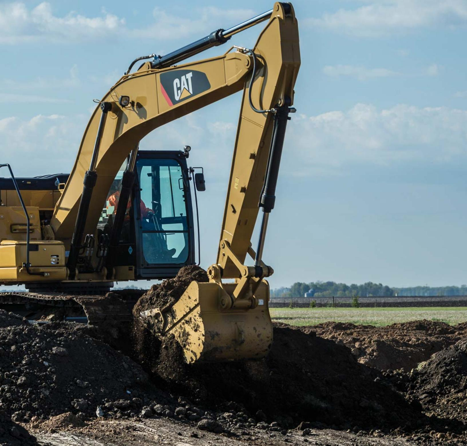
The new Cat 320F L is built for those who need strong, reliable performance at a low cost per hour. The machine features an efficient C4.4 ACERT engine that's light on fuel. It also has a proven hydraulic system that will help you take on a variety of tasks.
