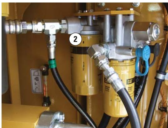
The drain filter (2) is one extra level of contamination prevention Cat excavators offer. Located in the pump compartment behind the pilot filter, the drain filter purifies the case drain from the main pumps, swing motor, and travel motors – all to enhance the life of the pumps and motors and increase uptime for you.
