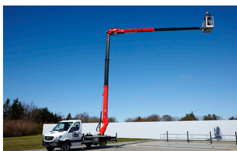
'Up and over' reach: 11 meters up and 12,5 meters out
